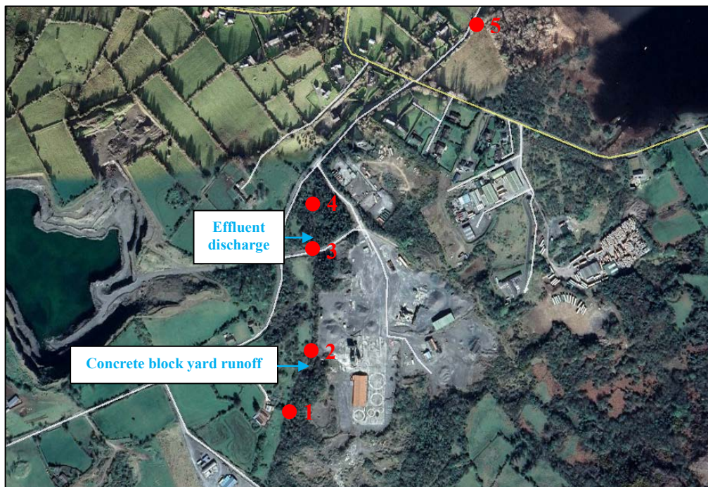
Figure 1: Location of biological assessments, yard drainage area and effluent discharge point, along the Aghamore Stream.
