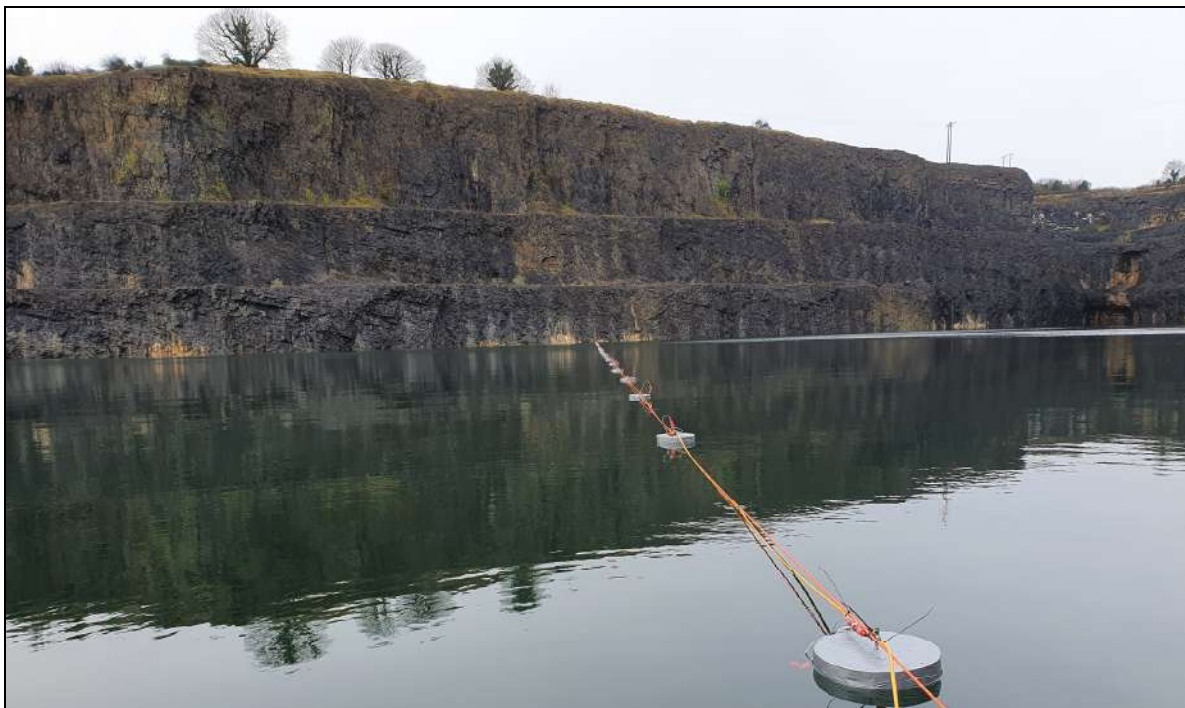
Fig. 2.10 Floating electrode ERT survey Area A.
